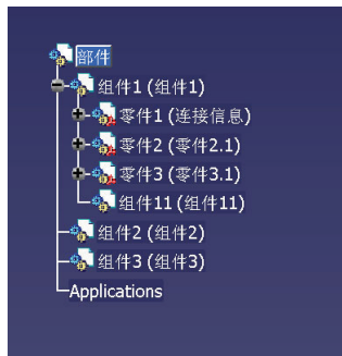
图1 MBD中装配层次关系的表达 Fig.1 Expression of assembly hierarchy in MBD
